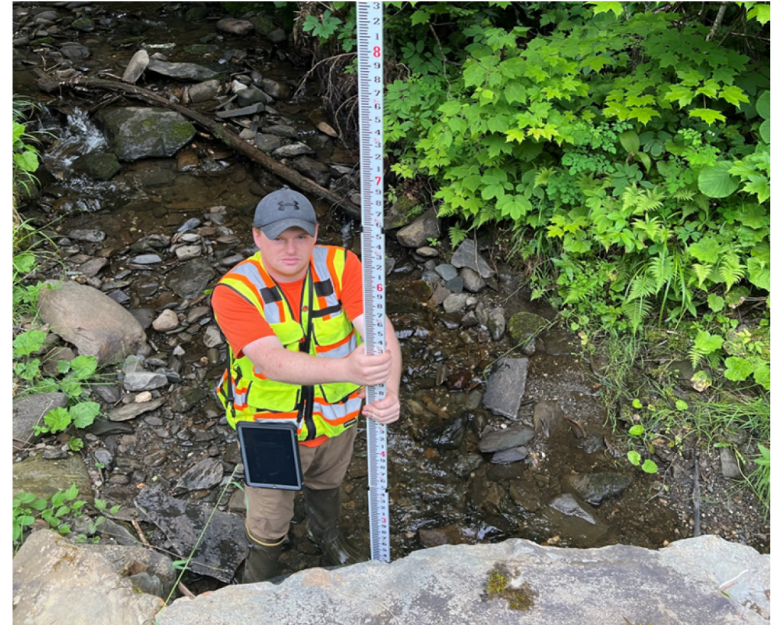
Pictured above: Aurora Summer 2024 intern, Dalton Rancourt, completes measurements for stream crossing condition and ecological suitability on one of the many structures conveying water throughout the Connecticut Lakes property's watershed. His work has been used to inform geomorphic compatibility and aquatic organism passage ability for the NH Stream Crossing Initiative.
